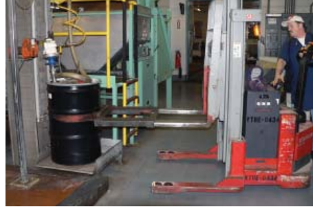
This stacker is fitted with a special drum-handling attachment.
