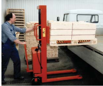
This stacker is well suited for moving loads up to 3,000 pounds for short distances.
