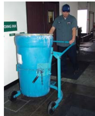
This drum dolly lifts and transports drums.
