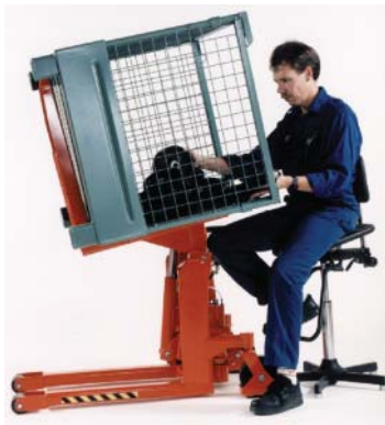
Powered tilters provide better access to large containers.
