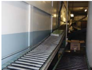
Gravity-activated conveyors work well for short, downhill runs.
